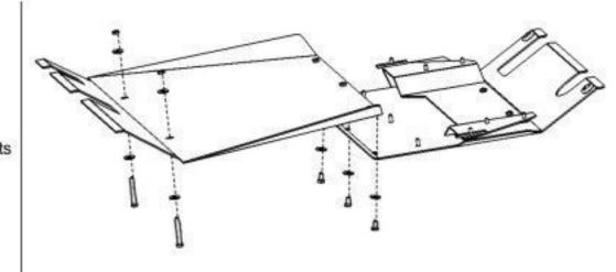
5. Joint the front part of the element "3" with element "2" using fastening slat and bolts M 10x20.
