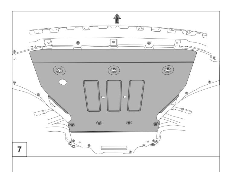
Engine bay and transmission elements skid plate has been designed and manufactured by LLC Metalloproduktsia. Product conforms to TOR 4591-001-25888788-2006 requirements. Product design is protected by model copyright certificates №89059, 15980, 15981, 15982, 15983. Patented in Russian Federation. INSTALLATION: Engine bay and transmission elements skid plate has been designed particularly for a certain vehicle. It should be
