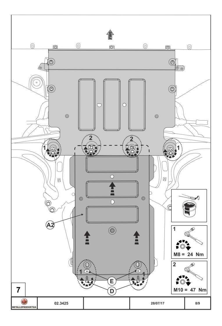
Engine bay and transmission elements skid plate has been designed and manufactured by LLC Metalloproduktsia. Product conforms to TOR 4591-001-25888788-2006 requirements. Product design is protected by model copyright certificates №89059, 15980, 15981, 15982, 15983. Patented in Russian Federation. INSTALLATION: Engine bay and transmission elements skid plate has been designed particularly for a certain vehicle. It should be
