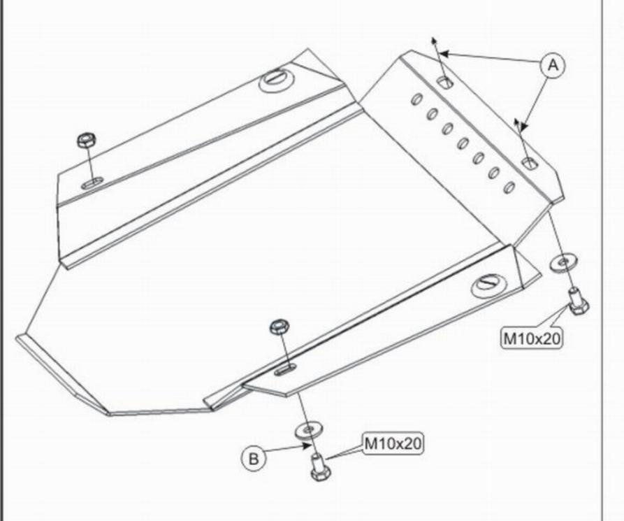
Mount this skid plate only after the skid plate for engine bay is Installed.
